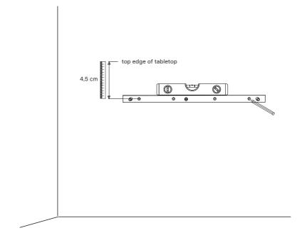
Move the bracket from the wall. Use a power drill to pre-drill the four holes at the marked points on the wall. Insert wall plugs (C) into the holes.
