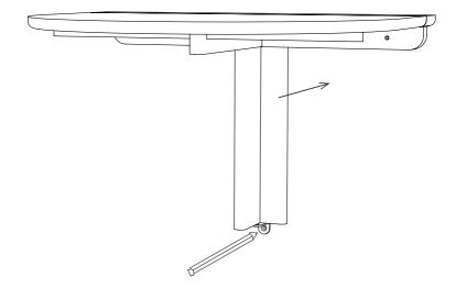
Move the table away from the wall-mounted bracket. Use a power drill to pre-drill the hole at the marked point on the wall. Insert a wall plug (C) into the hole.
