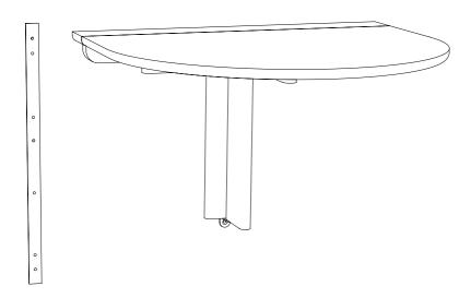
Position the bracket against the wall where the table will be mounted. Measure the desired height of the tabletop from the floor and use a pencil to mark the wall through the holes in the bracket. Ensure the bracket is level by using a spirit level.
