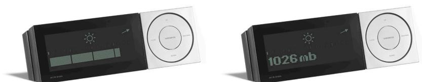
**Features:** Measures the barometric pressure in mb/hPa and indicates the pressure trend. A weather forecast is shown by symbols. Memory for maximum and minimum values registered. Two options for the display: Bar chart or actual digits.
